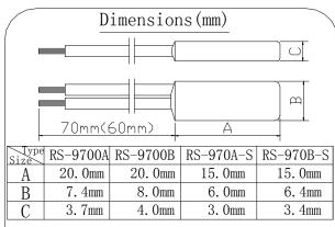
Notes: The lead wire can be made according to the customers' requirements. The above dimension is the one non-insulated sleeving.
