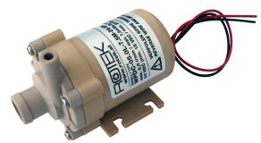
Thanks to the all-plastic construction (without bronze, stainless steel, or aluminum), the pump offers high resistance and is suitable for a variety of media such as demineralized water and solvents. The materials used include polypropylene and Peek, while the seal is made of silicone. Due to these materials, the pump is also conditionally resistant to alkalis and acids.
