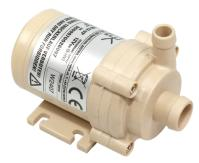
Thanks to the all-plastic construction (without bronze, stainless steel, or aluminum), the pump offers high resistance and is suitable for a variety of media such as demineralized water and solvents. The materials used include polypropylene and Peek, while the seal is made of silicone. Due to these materials, the pump is also conditionally resistant to alkalis and acids.
