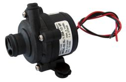
Thanks to the all-plastic construction (without bronze, stainless steel, or aluminum), the pump offers high resistance and is suitable for a variety of media such as demineralized water and solvents. The materials used include polypropylene and Peek, while the seal is made of silicone. Due to these materials, the pump is also conditionally resistant to alkalis and acids.
