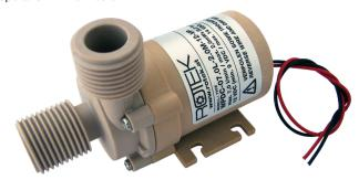
Thanks to the all-plastic construction (without bronze, stainless steel, or aluminum), the pump offers high resistance and is suitable for a variety of media such as demineralized water and solvents. The materials used include polypropylene and Peek, while the seal is made of silicone. Due to these materials, the pump is also conditionally resistant to alkalis and acids.
